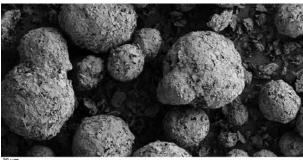
SEM micrograph: Grade CFA 250S
